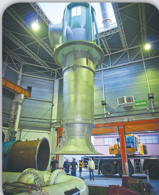
Flowserve offers a variety of products, such as this VCT vertical pump that could fill an Olympic-size swimming pool in less than three minutes.
